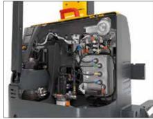
Sealed AC motor, controllers and connectors
